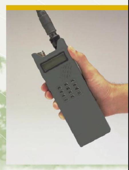
The TRC 5101 is a 2 W hand-held VHF transceiver which operates in simplex or half-duplex fixed frequency mode.
